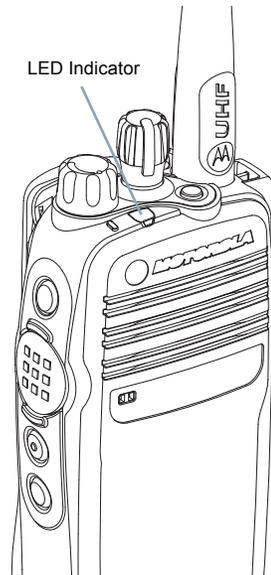
**Blinking yellow** – Radio is scanning for activity or receiving a Call Alert, or all local Linked Capacity Plus channels are busy.
